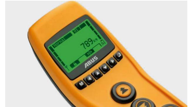
The **ABUS load indicator system** features a comprehensive range of switching and monitoring functions. The system offers an extremely short load detection time of only a few hundredths of a second, effectively protecting ABUS wire rope hoists against overloading. The measurement principle allows the load on the hoist to be limited without reducing the lifting height available.
