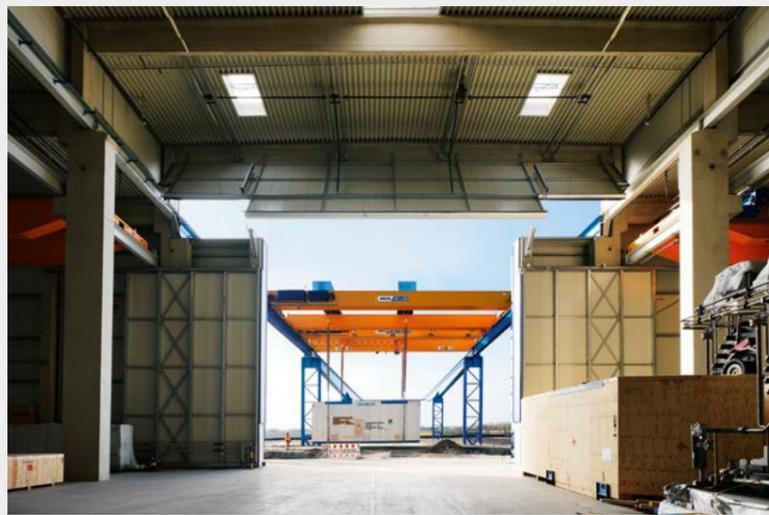
In the photographed application shown, the ABUS overhead travelling crane operates the crane flap, allowing the crane to travel back inside.
