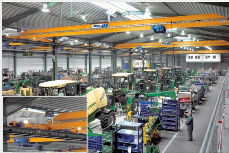
The ideal solution for a new factory: the ABUS ELK single girder overhead travelling crane with long angle chamfer adapted to suit the building haunch (version 3), optimising available height.
