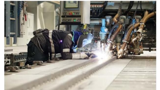
The moving portal welding unit designed in-house by ABUS personnel welds the web plates to the upper and bottom flanges and the rails on the top of the girder. The welding unit can complete up to eight welds simultaneously. The high-performance burners are automatically controlled by a PLC.
