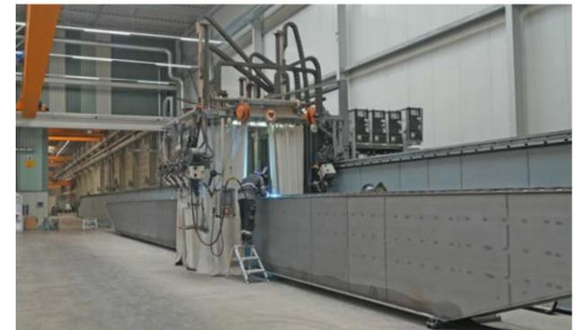
Following the welding of the closure plates and the installation of the end carriages, the paintwork required for the specific application is applied.
