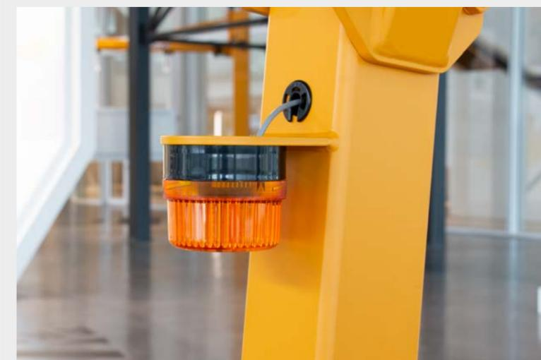
Highly visible flashing lights at operator level
