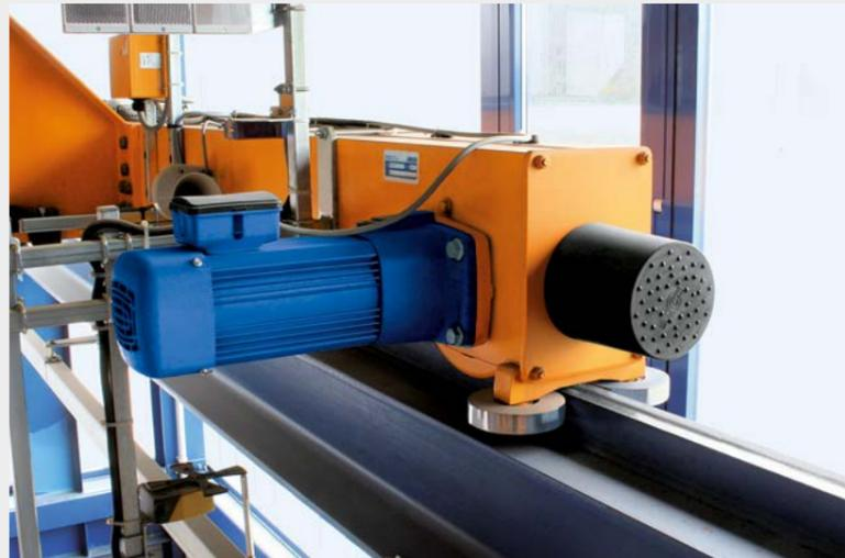
Optional twin hoist operation for for the transport of particularly heavy and bulky loads. The wire rope hoists are controlled from the crane control either individually or as a pair. A real safety advantage for your transport task.
