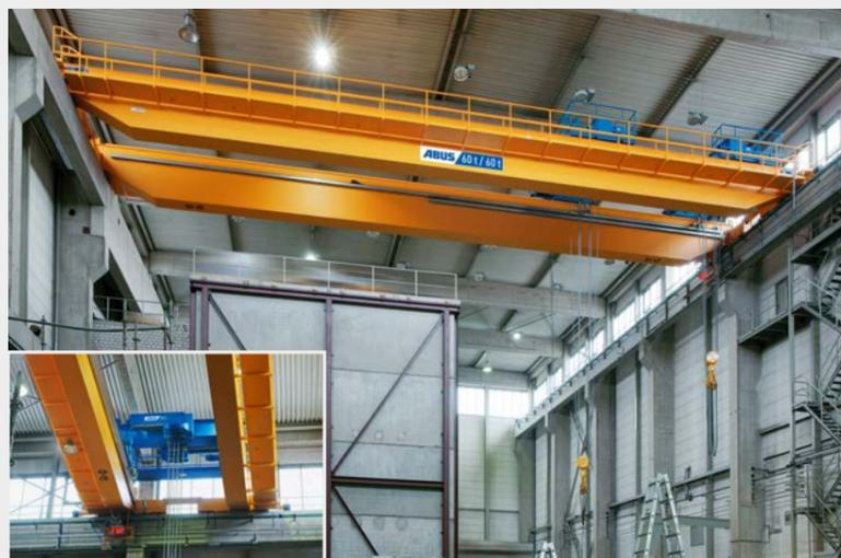
The end carriage may be mounted on eight wheels for even load distribution. Heavier loads can then be carried on a smaller crane track and the reinforcement otherwise needed in existing buildings may not be required.
