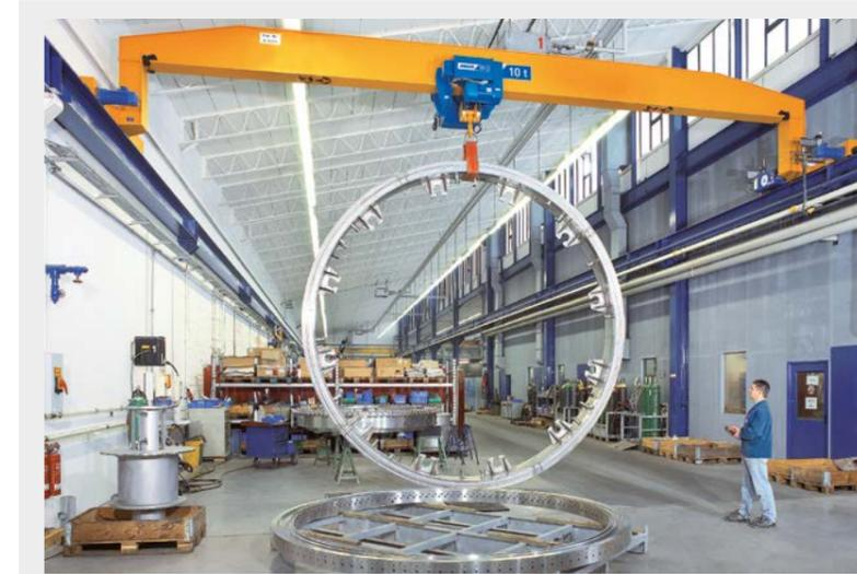
Stooled up crane bridge configurations are the ideal solution for special situations and buildings with difficult conditions.
