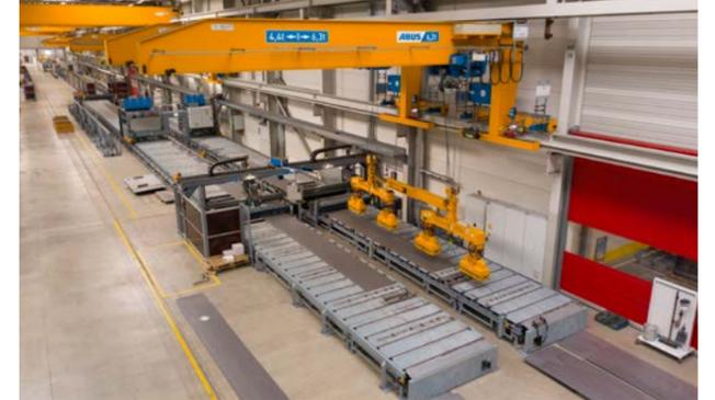
Before the next processing stage, web plates are stabilised with welded on buckling stiffeners. Following assembly on the box girder line, the box girder is ready for processing by the portal welding unit.
