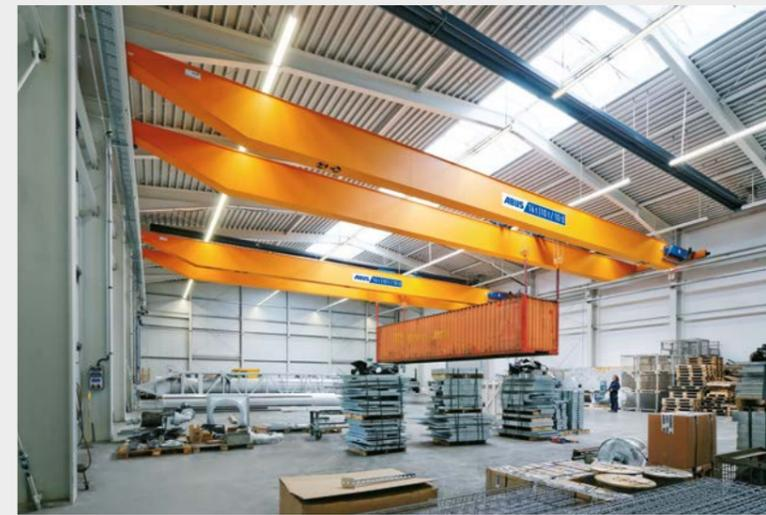
When transporting long and bulky goods, two adjacent cranes work in parallel to provide one risk-free load movement.
