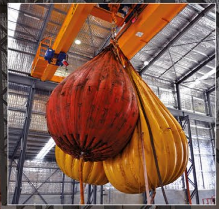
100t load test with water bags as test weights
