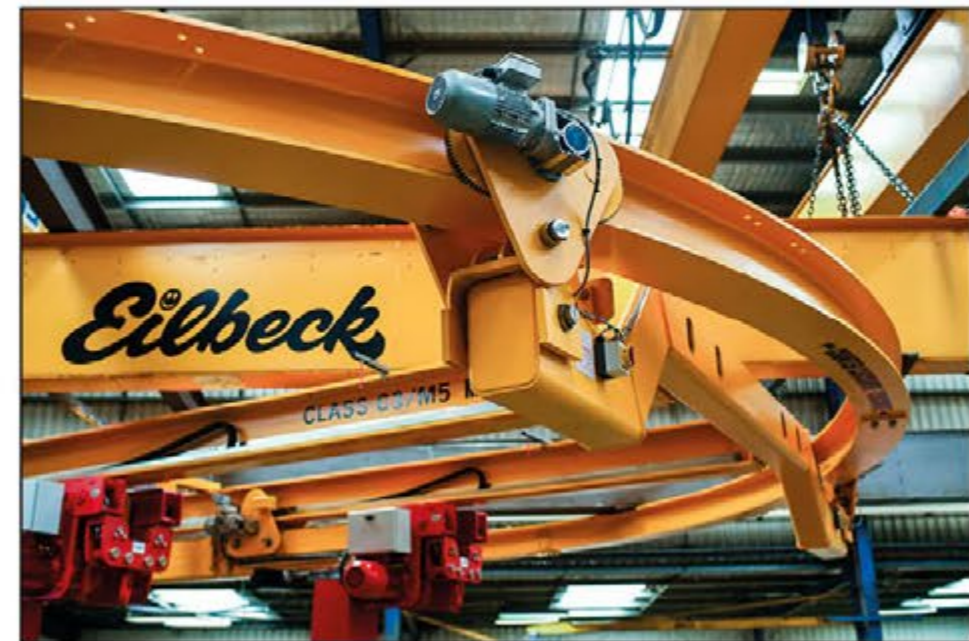
Hoists travel synchronously while maintaining 10(5+5)t MRC and independently maintaining 5t MRC each
