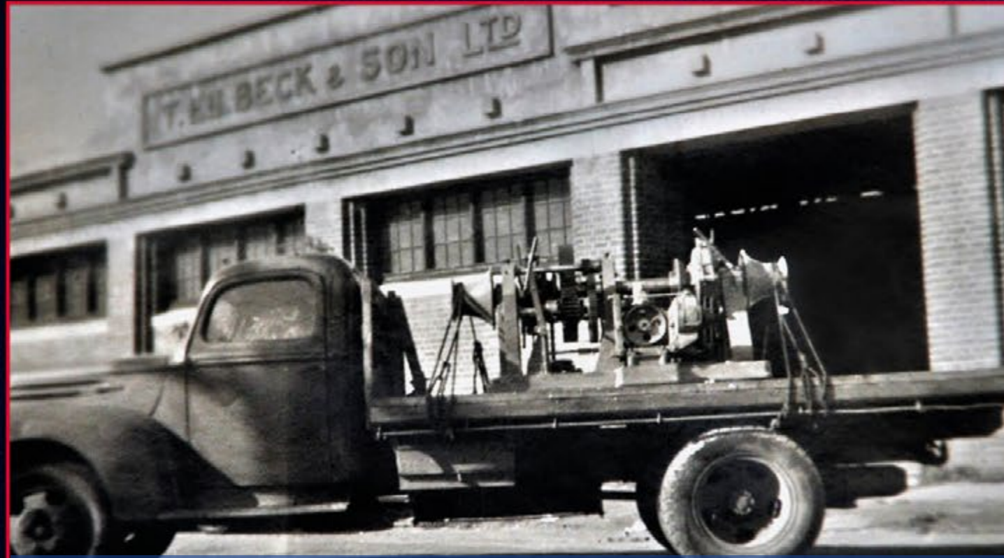
Early 1900's - Capstan Winch transported out of the Eilbeck's factory in John St, Perth
