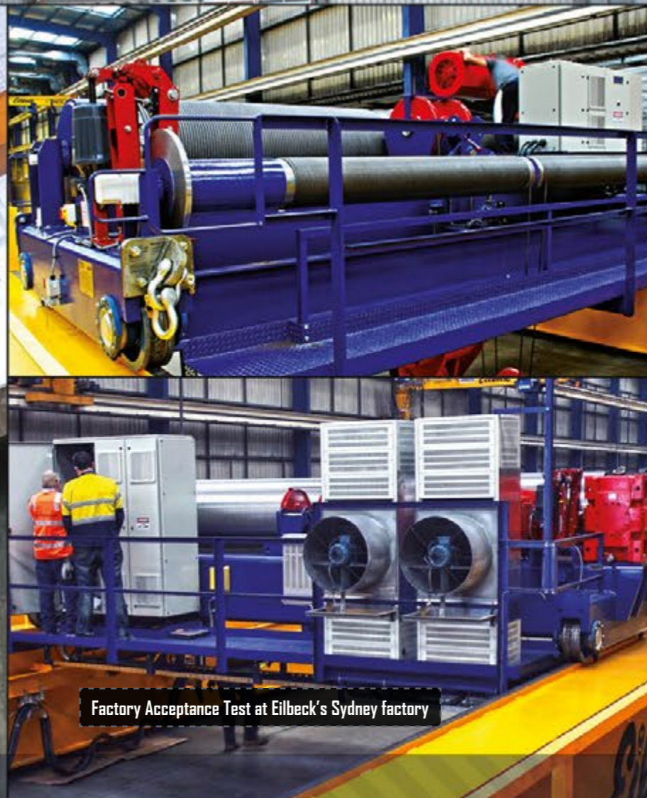
The crane at Trelawney site optimised for the 57m deep shaft lifting operations with separate settings for 100t (2.5m/min) and 40t lifts (17m/min)
