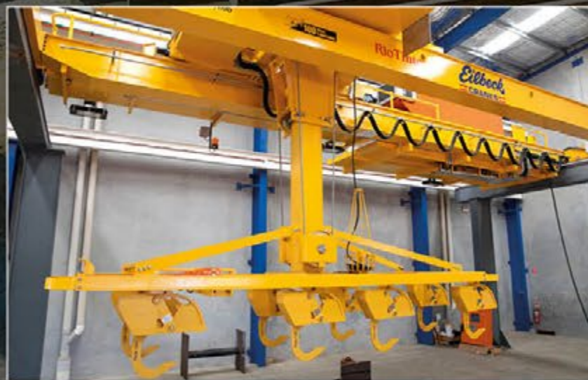
Self closing hooks for picking up to four wheel sets
