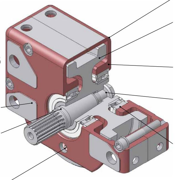
Wheel bodies and housing surfaces are blasted and undercoated. Plastic plugs protect all connection bore holes.
