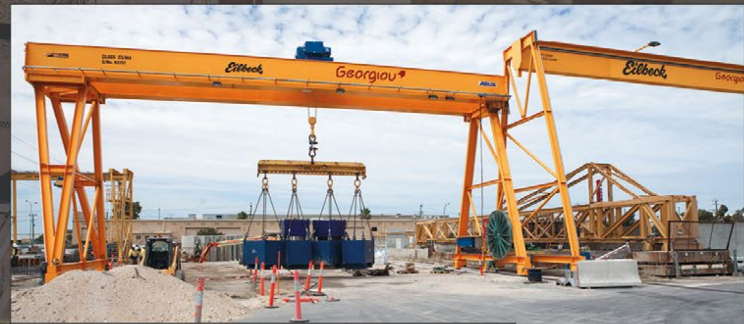
50t x 28m FPZLK (left) and 25t x 28m FPELK (right) - Georgiou Precast, Hazelmere Workshop WA
